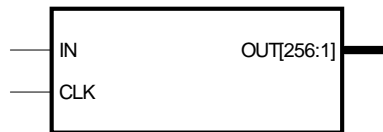
Figure 4.7: The 256-bit shift register macro.
